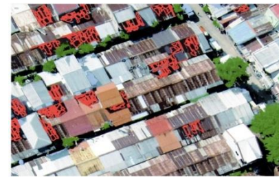
Fig. 8. Shadows are segmented and classified as separate from the structure objects.
