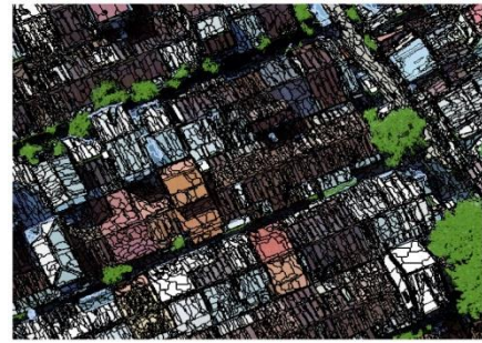
Fig. 7. Vegetation (green) and shadows (black) are classified (The rest are classified under surface)
