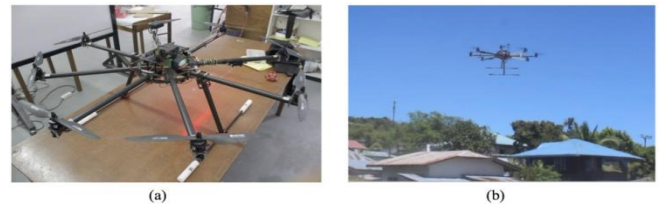
Fig. 3. (a) octocopter developed at the Center for Robotics and Automation, (b) actual operation
